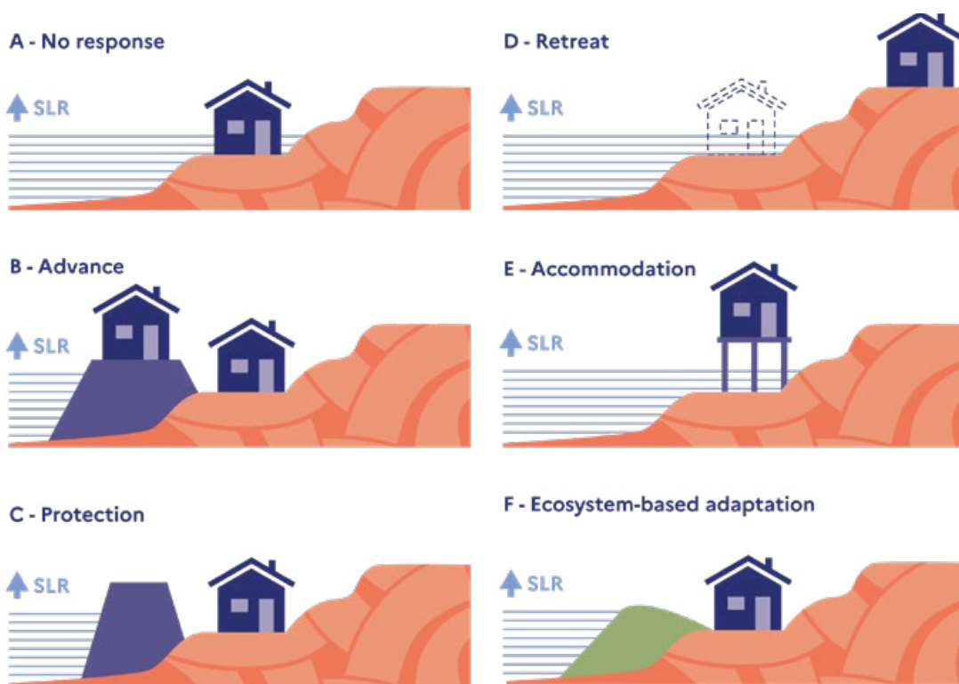
Typologie des réponses du Giec - Source : 2019, IPCC, SROCC, Box 4.3, Figure 1. Different types of responses to coastal risk and sea level rise (SLR*)
